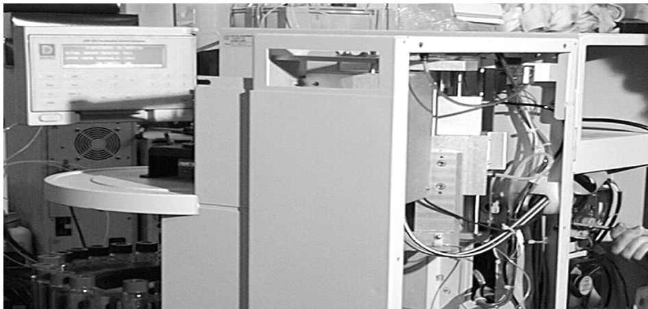
Figure 5-6. Accessing the Hydrocarbon Sensor
